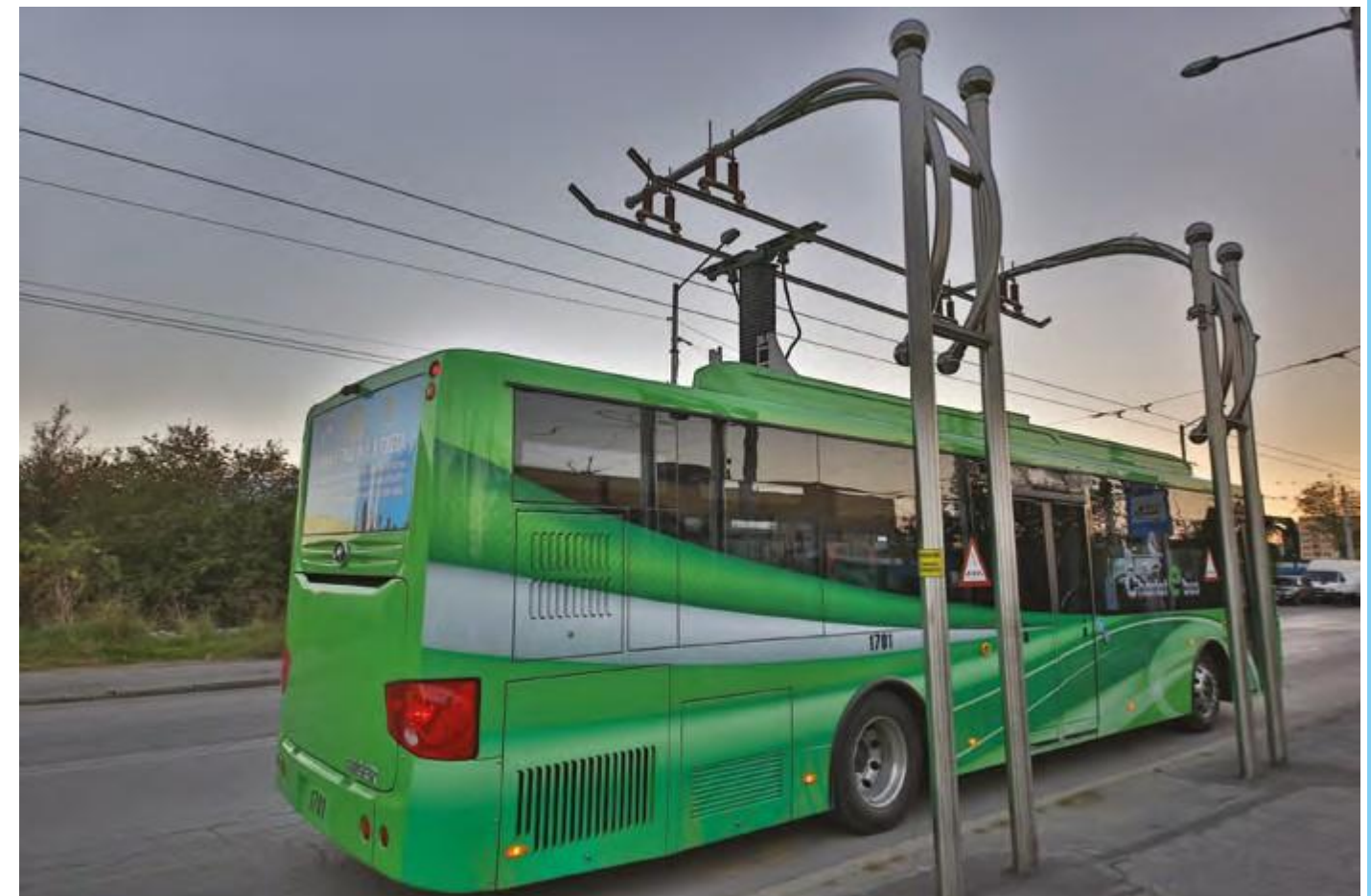
The pilot project with ultracapacitor electric bus in the capital was launched in 2014. The green model e-bus, photographed during its charging
